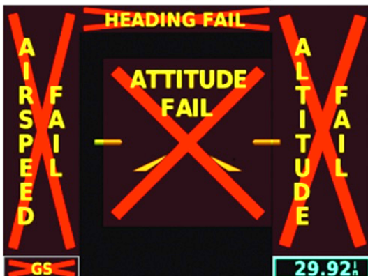
G5 ADI Failure Indications
