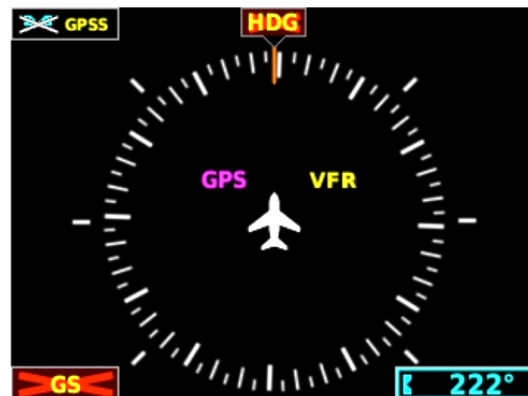
G5 HSI Failure Indications
